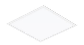
Pline panel light is a direct backlit lighting product with high lumen efficiency. It makes full use of all light and is more cost-effective compared with side lighting LED panel light. It adopts a high 130 Lumen per WATT 2835 SMD light source, the optical lens provides a uniform light output. It has an integrated iron plate, providing great thermal management. The micro prism diffuser provides anti-glare light effect.
