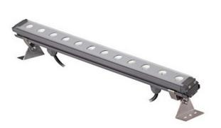
Ledbar 12×1.5W RGB architectural linear wall washer, small. Comes with the option of a 500mm lens hood. In a grey die casted powder coated aluminium with 4mm tempered glass. 24 Volt DC, ROHS compliant & CE certified.
