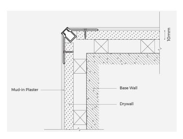
Model NoNL\_HC\_BRIM2727\_PROFILEMaterialAL6063-T5Surface<br/>ProcessingAnodizingDiffuserOpal PolycarbonateLight<br/>Transmittance>55%
